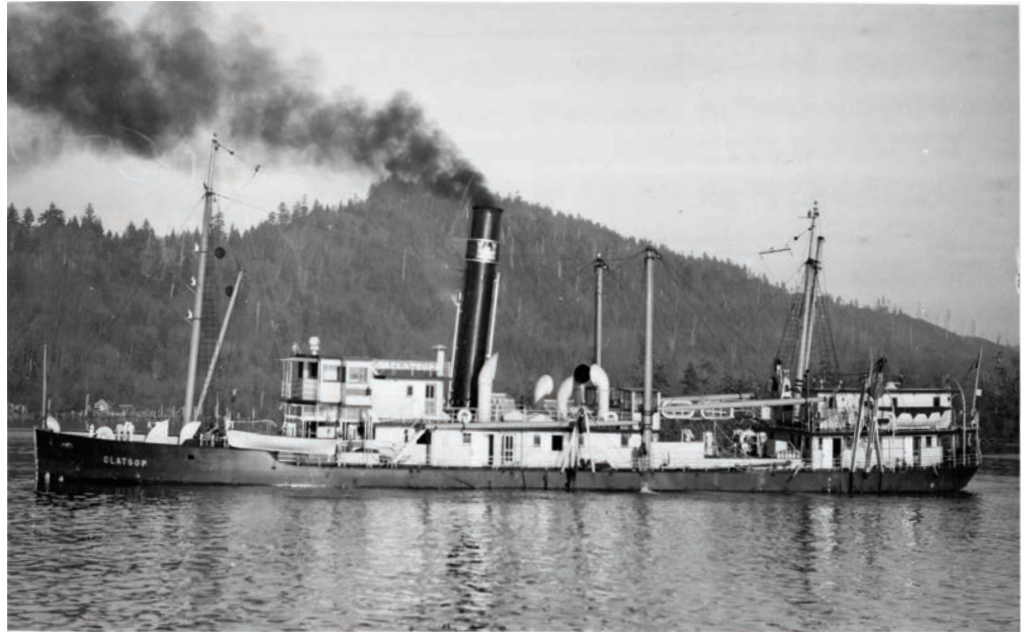
The seagoing hopper dredge Clatsop , circa 1938, doing maintenance dredging at the Skamokawa Bar on the Columbia River.
