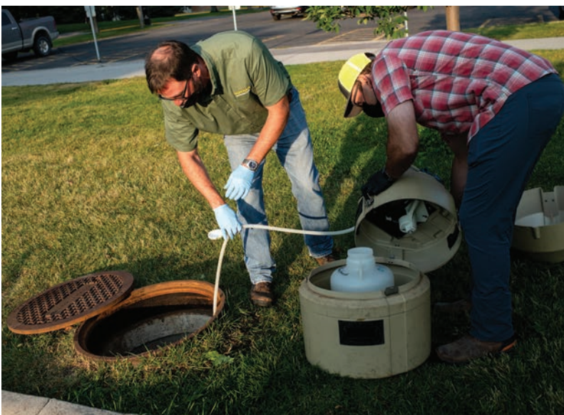
City of Bozeman Wastewater Pretreatment Coordinator Mark DeWald, left, and Water Reclamation Facility Lab Foreman Josh French, right, separate the housing unit of an autosampler to collect a wastewater sample jug from a Montana State University sewage line collection site. Mike Greener / HCN
