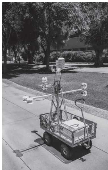
Ariane Middel is a climate scientist at Arizona State University whose research is offering a deeper understanding of the impacts of heat on the urban environment (top). MaRTy is a heat-sensing robot that helps Middel measure the Mean Radiant Temperature (MRT), or how humans experience heat in a specific urban location (above).
